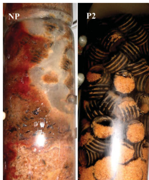
Figure 5. Photographs of the sludge bed of UAF NP and UAF P2.
